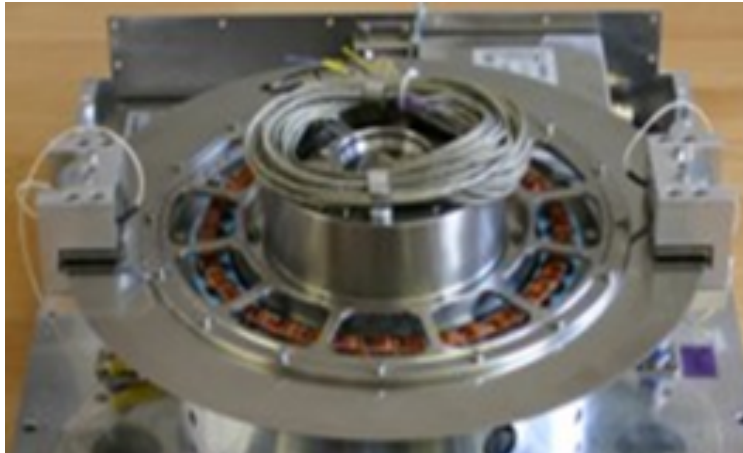
Figure 1 - 10 Nm Friction Disk Brake (MACCON)
